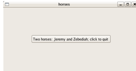
Figure 8.5.1 A window produced by the graphics toolkit GTK+. When the button is clicked, the window disappears.
